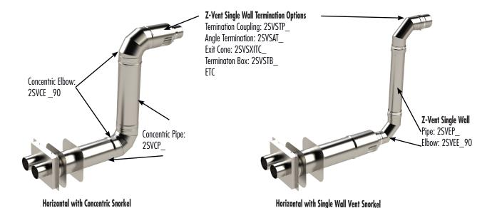
**Visit: Z-Vent Dimensional Data** for a complete list of concentric parts and single wall vent termination options.
